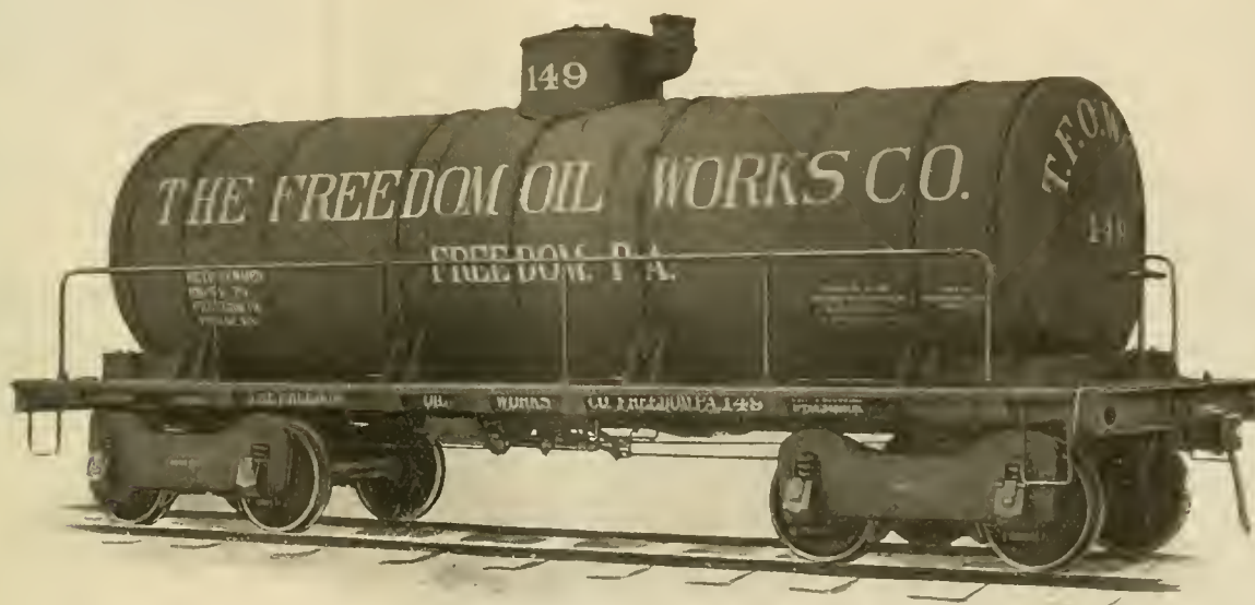
PRESSED STEEL TANK CAR. 7,000 U. S. GALLONS CAPACITY.
